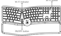
Step 2: Click the Wi-Fi button on the upper right corner of the keyboard to ensure that the position indicator of the Wi-Fi indicator light is flashing white.
